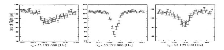
Cyclotron resonance at different values of the correction voltage
