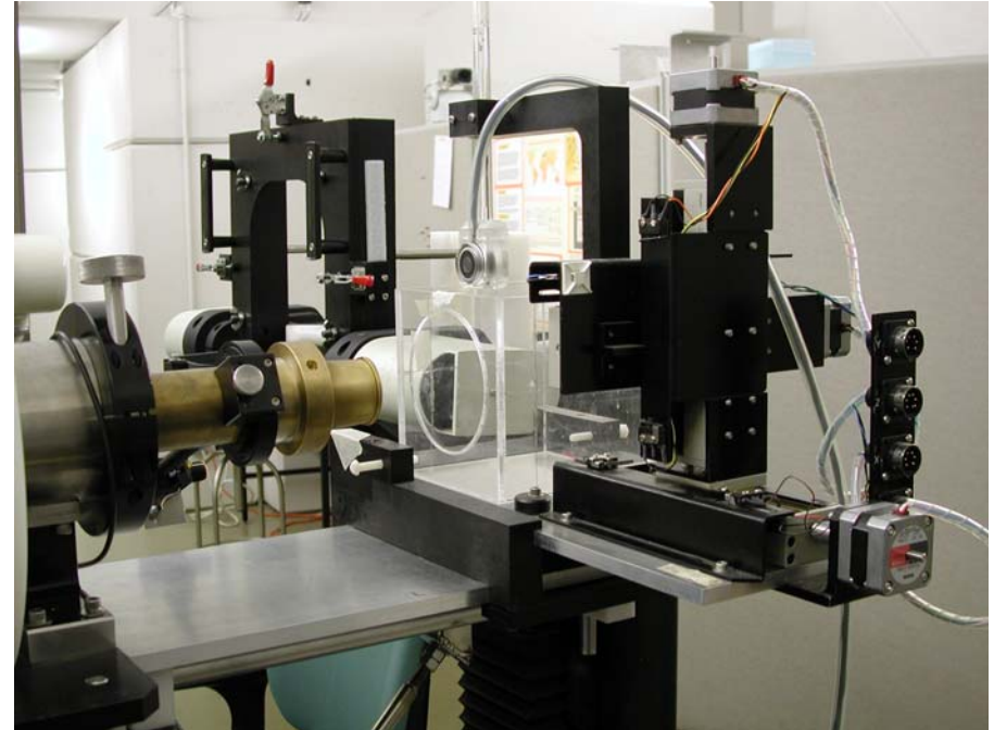
3D scanning table for dosimetry in a water box
