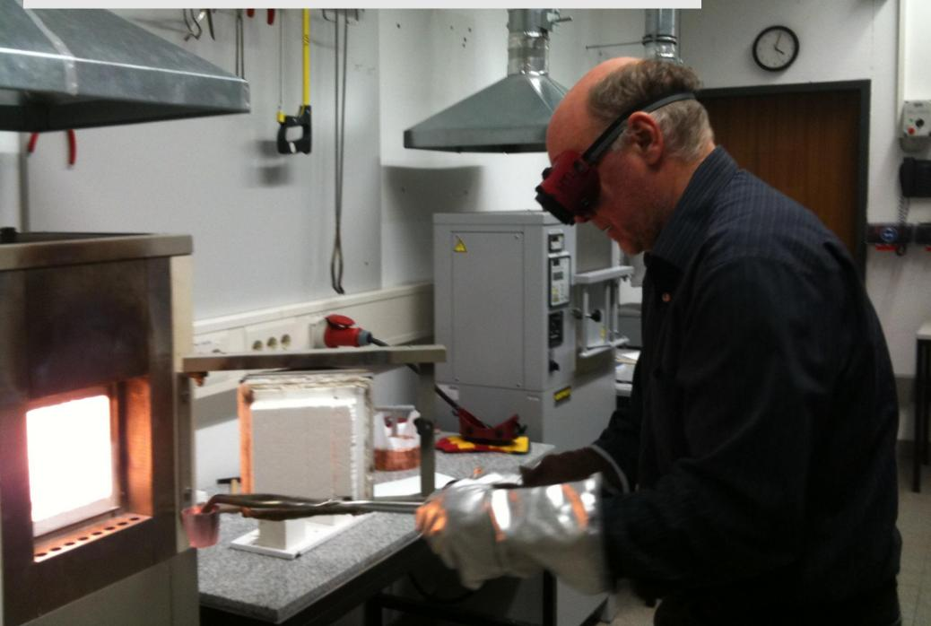
**NEW HIGH-T WEIGHT LOSS EXPERIMENTS Super-liquidus Conditions at T>1050°C for > 1hour**
