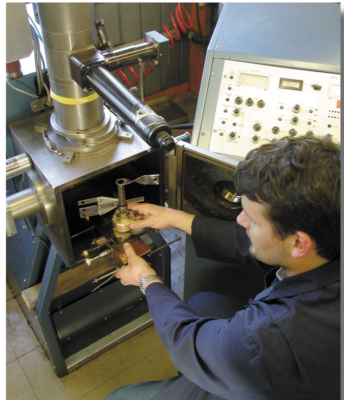
Positioning an ISAC target in the electron beam welder.
