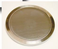
Electron beam welding of thin foil on isotope production target.
